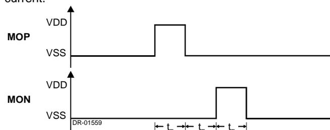
Figure 4: Motor drive on MON and MOP pins
